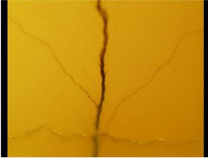
Typical channel of an electrostatic discharge. Note the branching off the main channel
