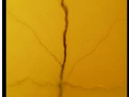
Typical channel of electrostatic discharge
