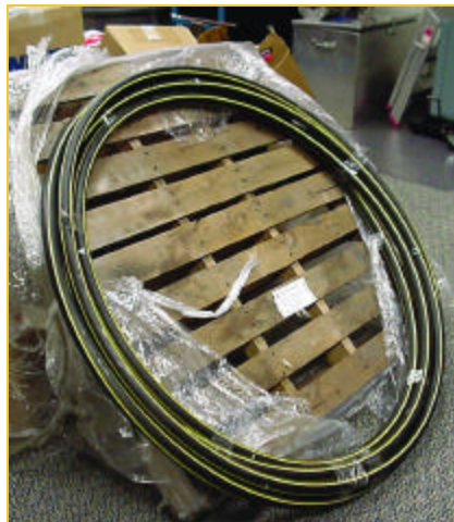
The pinholed pipe removed from the ground and coiled to be shipped back to Performance Pipe.
