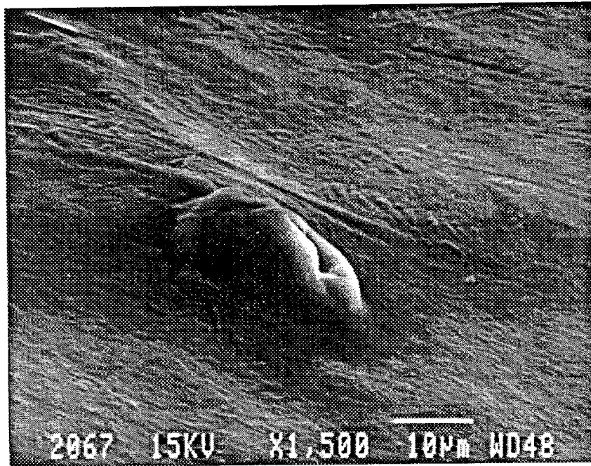
Figure 85. Features of pipe sample suggest local melting and resolidification
