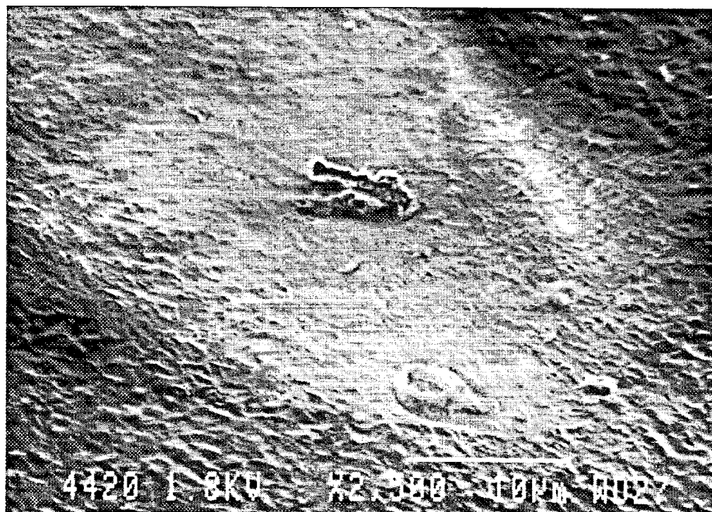
Figure 15. High-magnification view of leak site (2500X)
